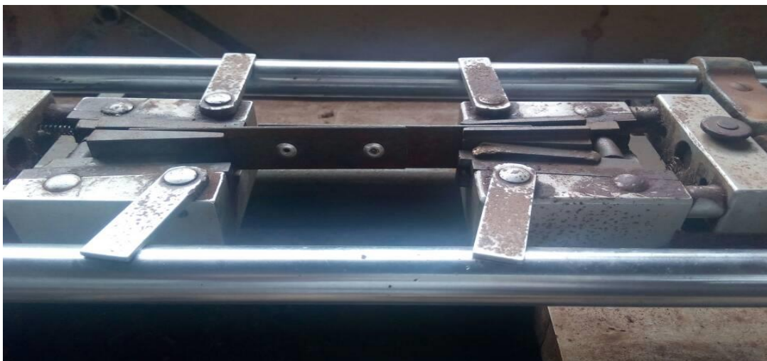
Plate 7: Mild steel lap joint during the test using Hounsfield Tensometer
