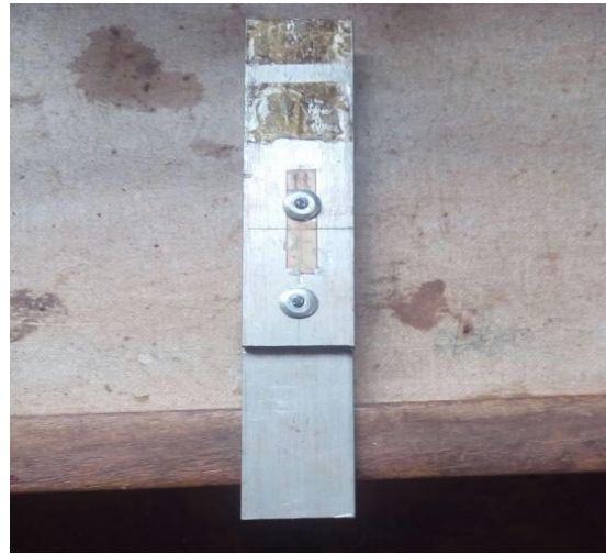
Plate 4: Riveted aluminium alloy lap joint
