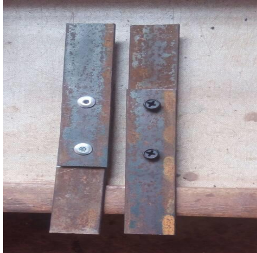
Plate 3: Riveted and bolted mild steel lap joint
