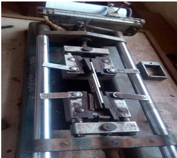
Plate 6: Aluminium alloy lap joint during the test using Hounsfield Tensometer
